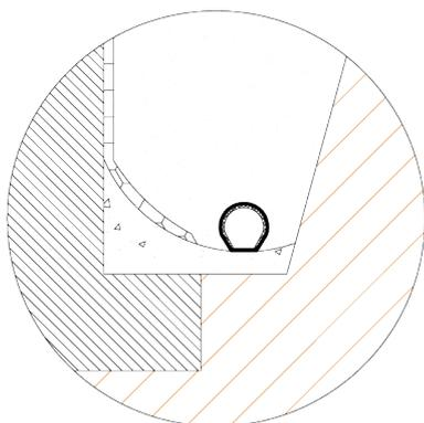
**FIGURE N°6 : COUPE DE PRINCIPE D'UN ACCOTEMENT & D'UNE CUNETTE**
