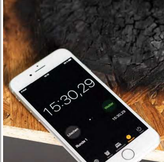
15-minute exposure to flame only chars surfaces.
