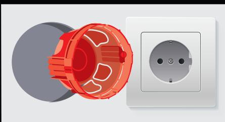
Standard stipulates that all flush-mounted electrical circuits must use flush-mounted boxes to comply with the following requirements.
